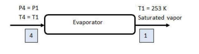
Heat extracted by evaporator
