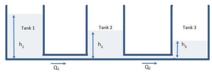
The flow is opposed by pipe friction, and the level of liquid in each tank oscillates to an equilibrium. Differential equations that describe the dynamic change in liquid height in each tank and a momentum balance are solved numerically.
