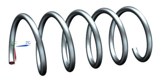
The design variables are the diameter of the wire d, the outside diameter of the spring D, and the number of coils N.
